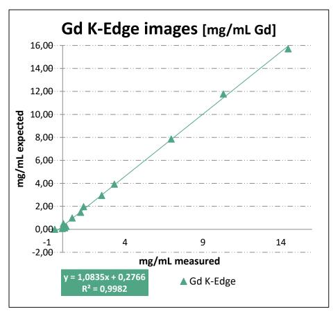
These graphs show the correlation between <u>expected concentrations</u> (densities) to the <u>measured concentrations on SPCCT for Gadolinium</u> using kedge imaging.
